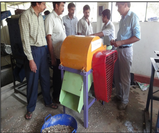
Photo 3: Areca sheath shredding machine
